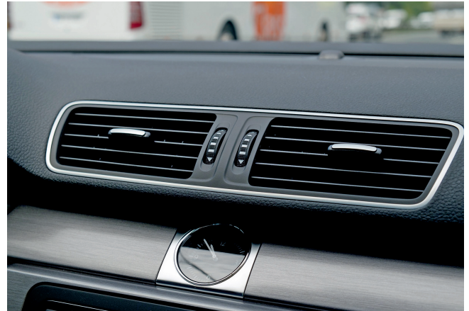
Fig. 5. The semi-aromatic PA of the Leona SG range from Asahi Kasei permits high-quality surfaces to be achieved without special treatment. © Asahi Kasei
